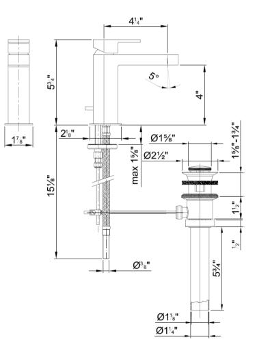
We cannot guarantee the accuracy of this information. Dimensions are nominal - for guidance only and are not to be used for pre-installation.
